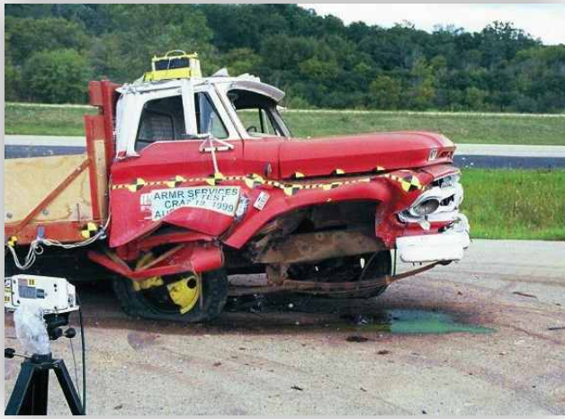
7-ton vehicle driving at 48 km/h, destroyed after impact with 3 bollards (under supervision of US State Department)
